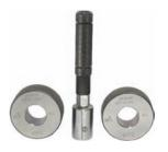
Air Plug Gauge with Setting Rings: Useful for internal bore size, taper and ovality measurement. Through or blind bore design. Special air plug for long bore, short bore and taper bore. Available with hard chrome plating for longer life in the range 4mm to 200mm.
