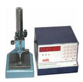
Useful for checking the diameter and length on standard comparator using LVDT and Digital Display unit having a resolution upto 0.1 microns with absolute display value and data can be transferred to PC for further analysis.
